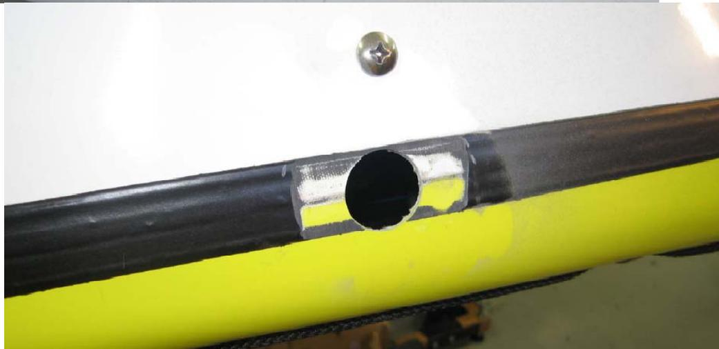
11. Clean the area with Denaturated Alcohol and install a fitting into the hole using Sikaflex-291 (a bead on the hull, starting a couple of mm outside the hole and going almost up to the flange diameter) slightly out + in when the fitting is tightened.
